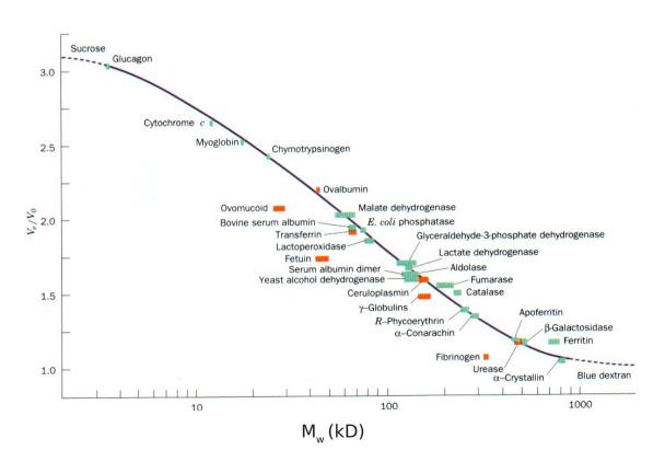
$V_t = V_x + V_o$ , where  $V_t$  is the total column volume,  $V_x$  is volume occupied by the stationary phase and  $V_o$  is void (remaining) volume
