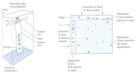
Resolving power can be readily improved by adding a second dimension using a second solvent system
