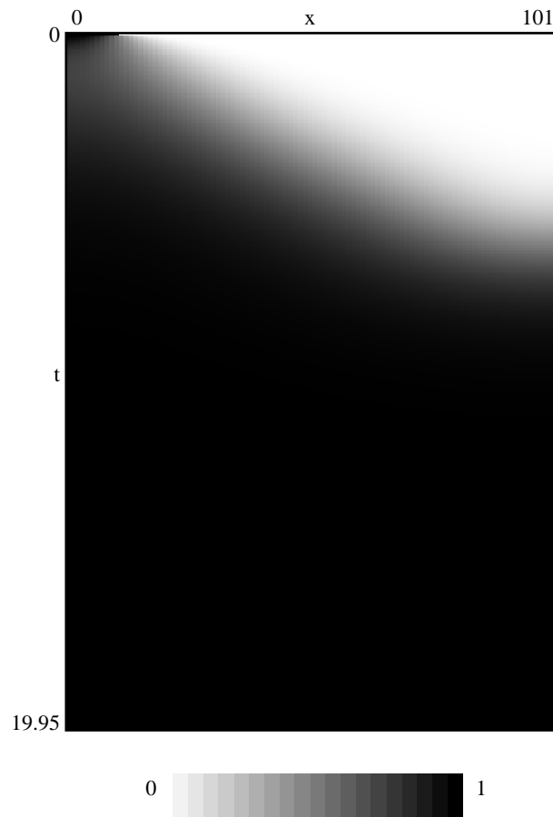
Figure 2: Space-time plot of the solution of the logistic reaction-diffusion equation. The details of the simulation are given in the text. The values on the x axis are actually indices into our pseudo-array rather than actual values of x . The latter are recovered by multiplying the indices by \Delta x .
