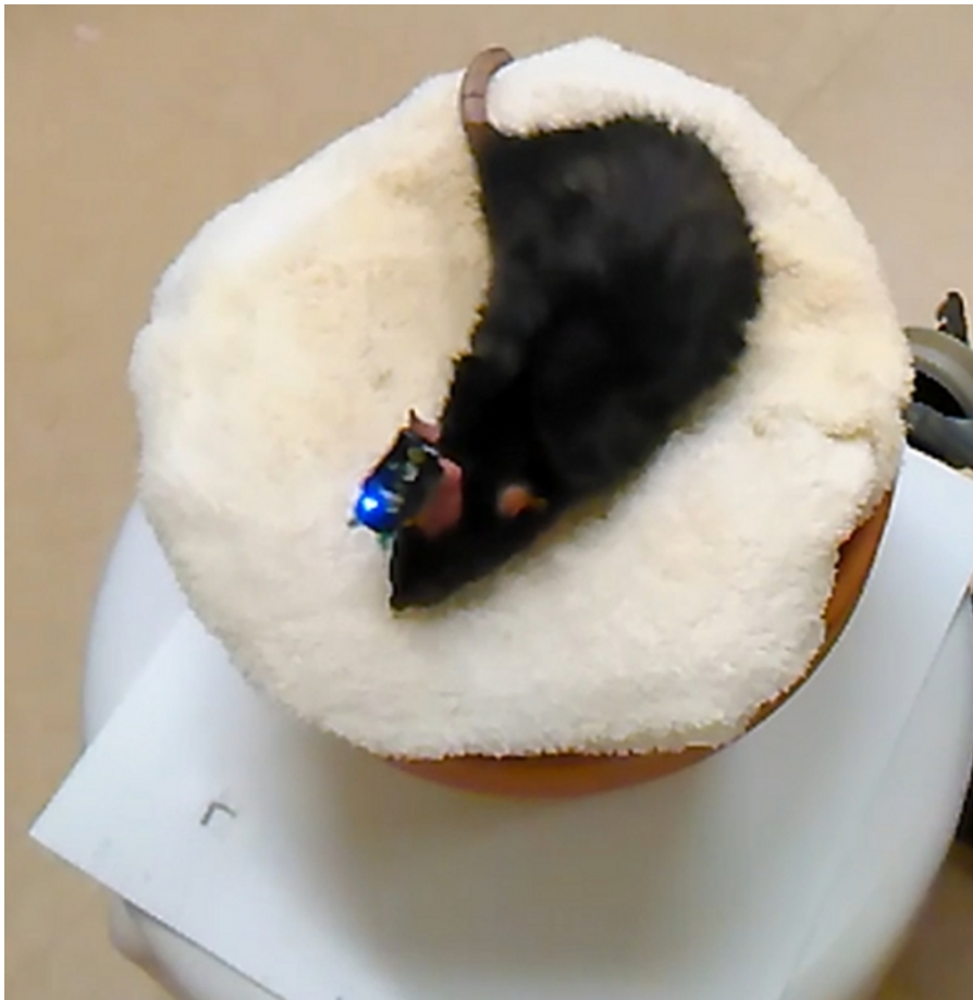
Figure 1: Photograph of a rat with the wireless head-stage (board with pre-amplifiers and a blue LED) attached to an implanted silicone probe. The probe is positioned under the dental acrylic (pink material) and is not visible. Please click here to view a larger version of this figure.
