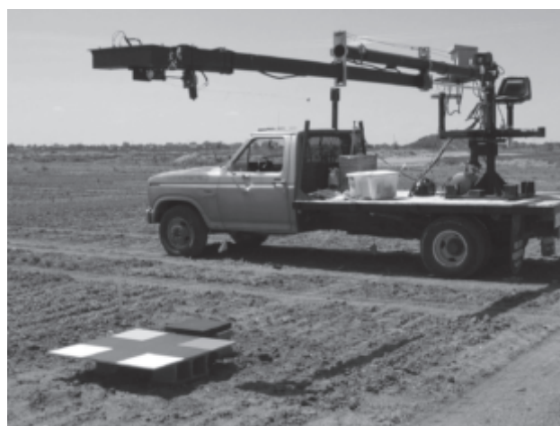
Figure 1. Flat-bed truck with sensor mounted on boom arm for image acquisition. A color version of this figure is available at the ASPRS website: www.asprs.org .
