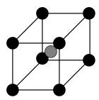
Note that in both cases, the shading is only intended to distinguish corner atoms from the others and is not intended to indicate different types of atoms.
