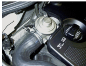
Photo 2 Remove the hose at the combination EGR shut-down valve housing to inspect for carbon buildup.
