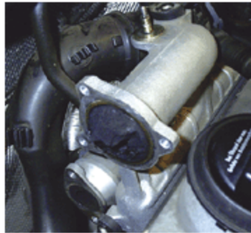
Photo 3 There is a significant loss of power when the intake is plugged.
