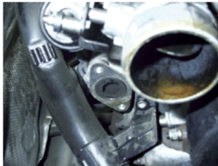
Photo 1 The EGR cooler (small flange below intake) appears to be where the problem starts.
