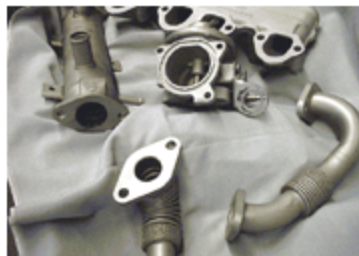
Photo 4 Ultrasonic cleaning works the best to restore "like-new" performance.
